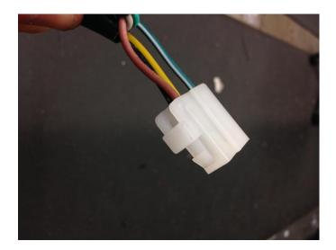
**Step 2:** Disconnect this connector, followed by removing the previous Baja Designs headlight, horn, flasher, and turn signals. Mount these components to the new Squadron headlight in the same manner.
