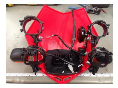
**Step 3:** Locate the white three pin connecter that you found in Step one. Plug the three pin connector into the corresponding plug on the Skene dimmer. Do the same with the Baja Designs Squadron/S2 into the dimmer box.
